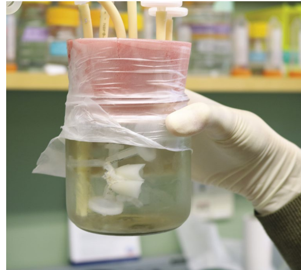
Top Left: Engineered rat lung during culture, growing inside a bioreactor designed to mimic physiological conditions.
