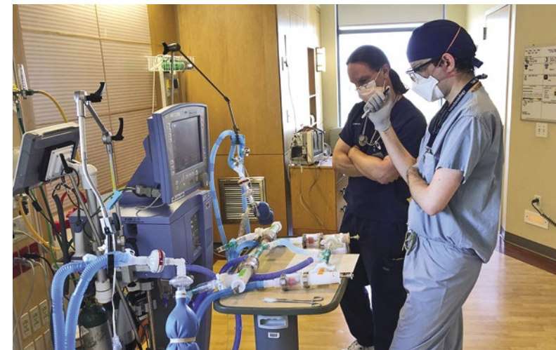
Left: Sam Brickman Raredon, a member of the Niklason Lab, illustrates how PReVentS can treat multiple patients at the same time. Middle: PReVentS being tested and analyzed. Top Right: A design that was easy for hospital staff to quickly assemble in a high-stress environment was critical. Right: CHIME members also designed an adapter to convert an off-the-shelf positive end-expiratory pressure ventilator valve element into a device that can be used in the vent-splitting circuit. Bottom: An alternative multiplexing design that incorporated Venturi-based pressure measurements for each air pathway.
