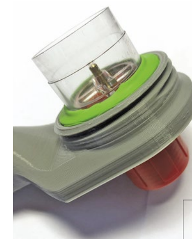
Left: Sam Brickman Raredon, a member of the Niklason Lab, illustrates how PReVentS can treat multiple patients at the same time. Middle: PReVentS being tested and analyzed. Top Right: A design that was easy for hospital staff to quickly assemble in a high-stress environment was critical. Right: CHIME members also designed an adapter to convert an off-the-shelf positive end-expiratory pressure ventilator valve element into a device that can be used in the vent-splitting circuit. Bottom: An alternative multiplexing design that incorporated Venturi-based pressure measurements for each air pathway.
