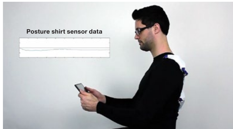
Above (l to r): Robotic skins are not exclusive to inanimate objects. They can also be applied to an upper body garment using its sensors to track human posture. Actuators pulse to inform the wearer that they should sit upright.
