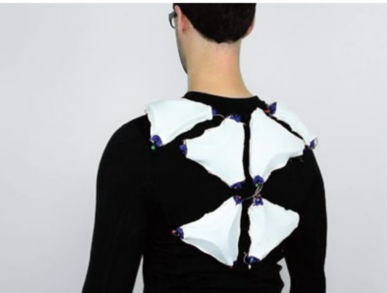
Above (l to r): Robotic skins are not exclusive to inanimate objects. They can also be applied to an upper body garment using its sensors to track human posture. Actuators pulse to inform the wearer that they should sit upright.
