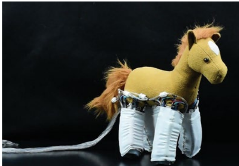
Left & Above: Inanimate objects — like a plush horse — can come to life and walk when wrapped with a robotic skin.
