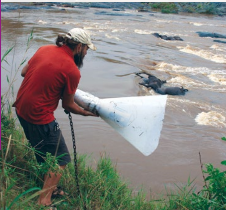
Left: Water sensor in hippo-proof sensor housing being deployed to Mara River; Center and Right: Ultrasonic depth logger positioned on bridge over Mara River
