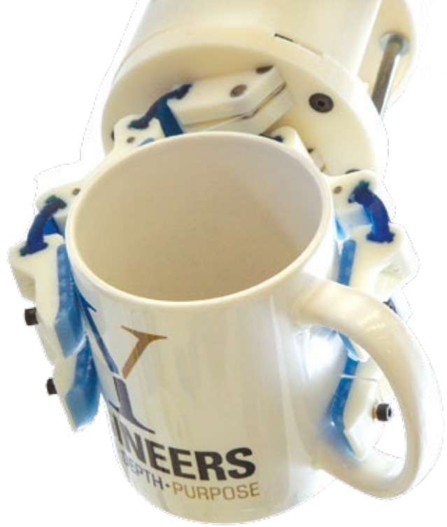
Grasping technique of underactuated robotic hand
